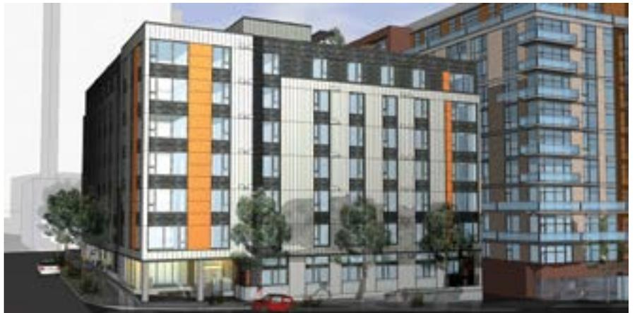
The 7-story, 145 unit structure utilized the unique modular steel framing system that was developed by IGB Systems. In this project, their steel framing system was installed over a 2-story partially below-grade, post-tensioned concrete parking garage.
